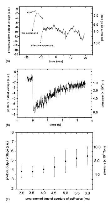
FIG. 3. Monitoring of the fast varying pressure inside vacuum chamber: (a) by setting the time of aperture of the puff valve to 5 ms, (b) after its filling and evacuation by vacuum system, (c) by varying the time of aperture of the piezoelectric valve of injection of gas.
