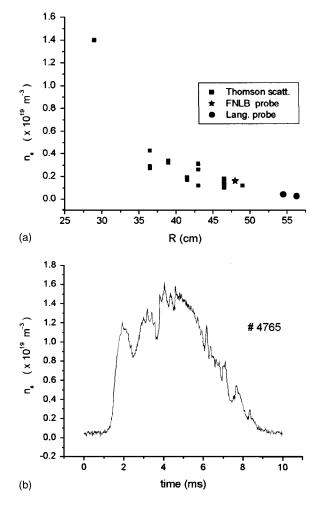
FIG. 4. Experimental measurements: (a) radial profile of the density in ETE measured by Thomson scattering, fast neutral lithium beam probe and Langmuir pobe, (b) temporal evolution of the edge density in ETE discharge (R=48 cm).
